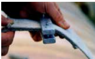
1. Feed each end of strap through the clamp plates.
