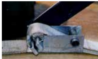
5. Fit spanners over the ends of the clamp and rotate to snug straps down.
